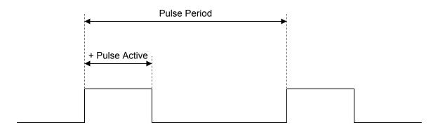
The pulse period may be a minimum of 2 ms to a maximum of 9999 ms. The pulse width is a minimum of 1 ms to a maximum of 9998 ms. If the pulse length command requests a length greater than the period, it is automatically reset to 1 ms.
